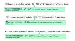
In the ASTRID project, we plan to increase the duration of the cycles (and hence the load factor) in 3 stages, represented in the diagram below:
