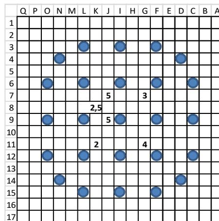
Fig. 1. Experimental UOX-5 cycles fuel pins in GRAVELINES.
