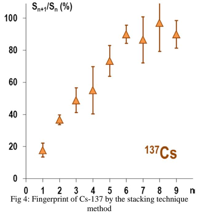
Fig 4: Fingerprint of Cs-137 by the stacking technique method
