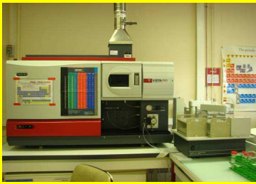
Seaspray nebulizer, cyclonic chamber, axial view, CCD detector
