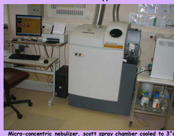
Micro-concentric nebulizer, Scott spray chamber cooled to 3°C with Peltier effect, DDEM detector
