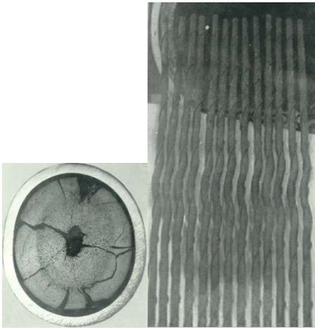
Fig. 8: Pin deformation.
