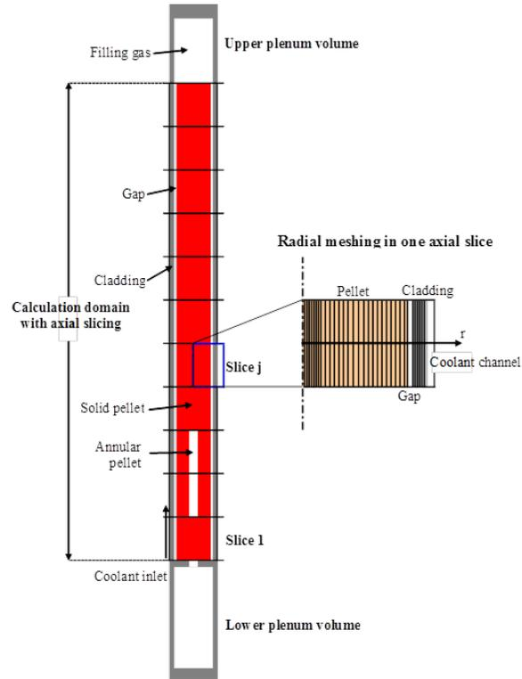
Fig. 5: Calculation model of the fuel pin.
