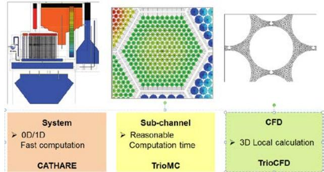
Fig. 10: Thermal-hydraulic simulation tools/ available modelling scales.
