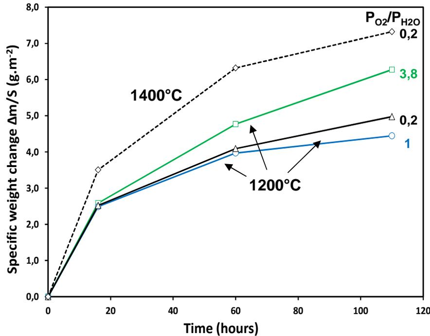
Global behavior resulting from the competition between simultaneous growth and volatilization of a silica oxide
