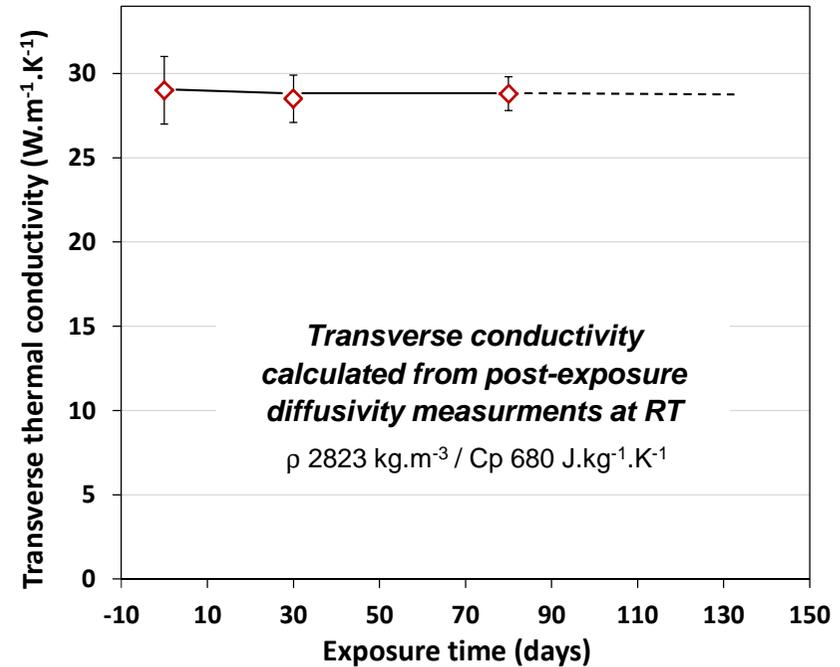
**No effect of oxidation on the thermal behavior after 80 days**
