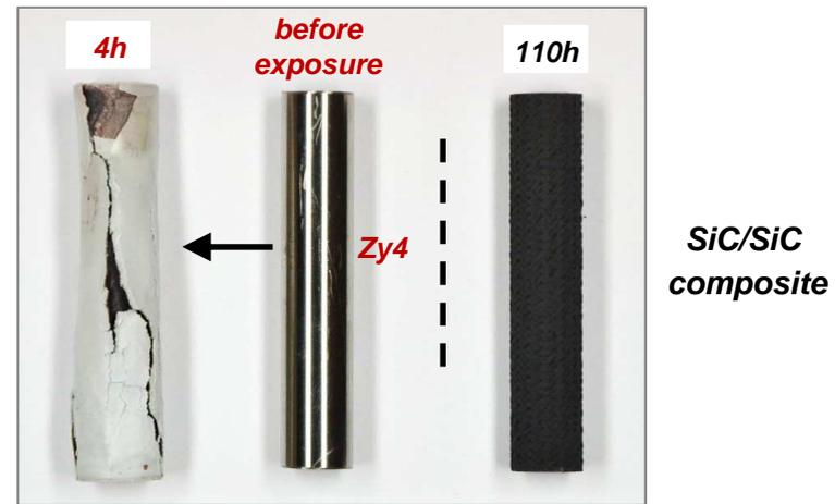
**Extremely slower oxidation kinetics of SiC/SiC than for Zr alloys !**
