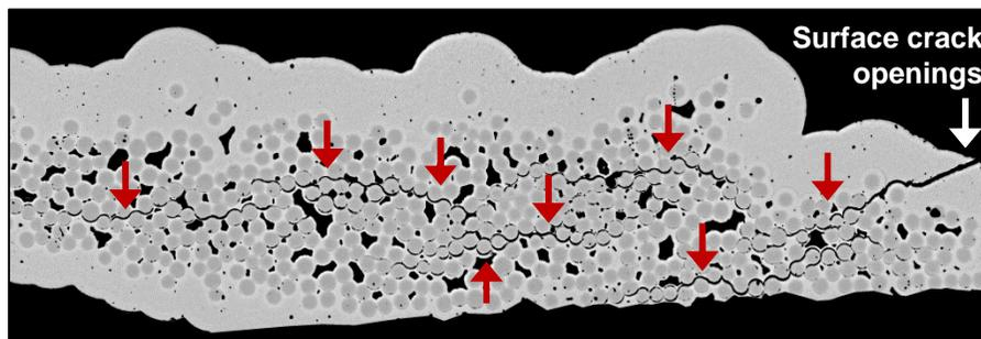
Water infiltrates through the larger crack openings and oxidizes the SiC materials from inside and not just on the surface
