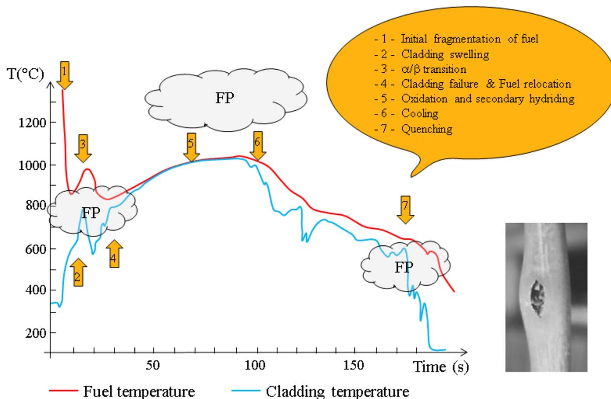
Figure 1: Different phases of a typical LOCA sequence.
