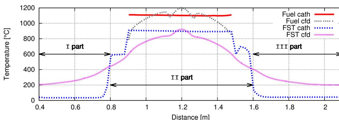
Figure 6: Wall temperature calculated with CATHARE and CFD.
