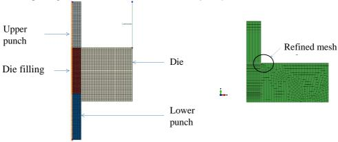
Fig 7: 2D geometrical axisymmetric model (left), Mesh tools (right); greatly improved mesh
