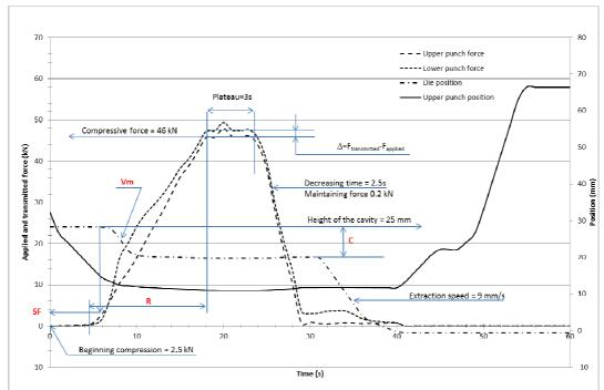
Fig 1: Compaction cycle used to shape annular pellets
