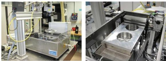
Figure 3: SLM demonstrator used for the process parameter search
