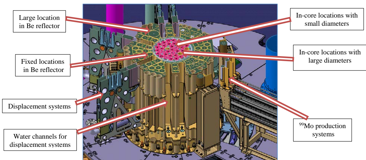
Figure 3: Irradiation locations in JHR core and reflector (schematic cross-cut)
