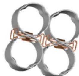
fuel rod spacers (SS, Ni alloy)
