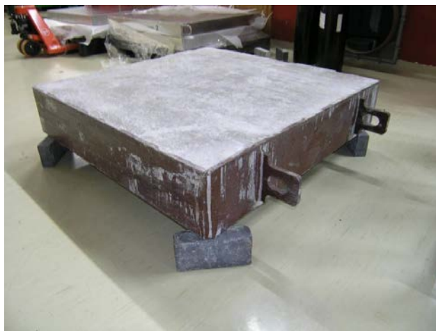
Figure 1. Concrete shield block.
