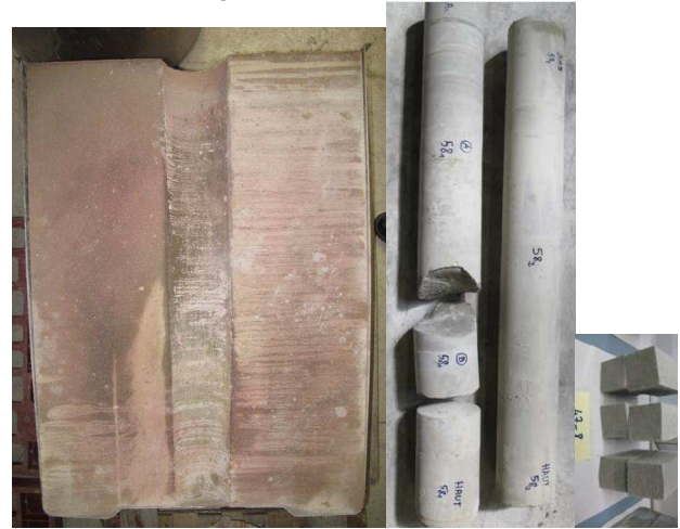
Fig. 10: 380 liter package cross-section and samples
