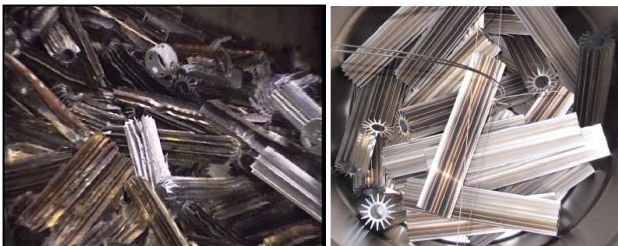
Fig. 3: (Left) real scrap magnesium waste (Right) simulated magnesium waste
