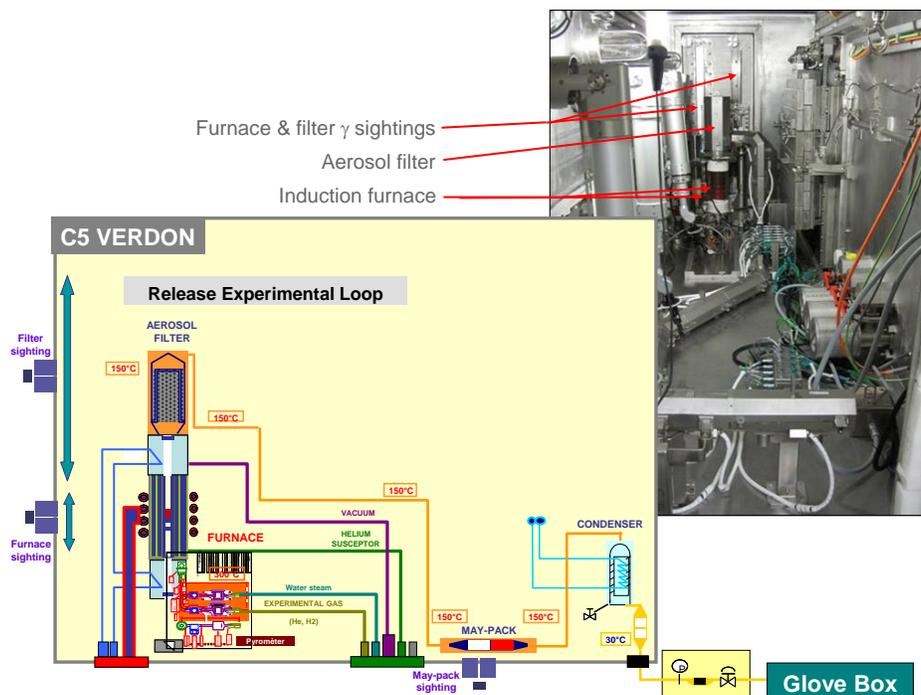
Figure 2: The so-called release experimental loop (CER)
