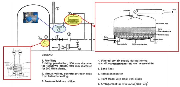
Fig. 1. General diagram of the FCVS in French PWRs
