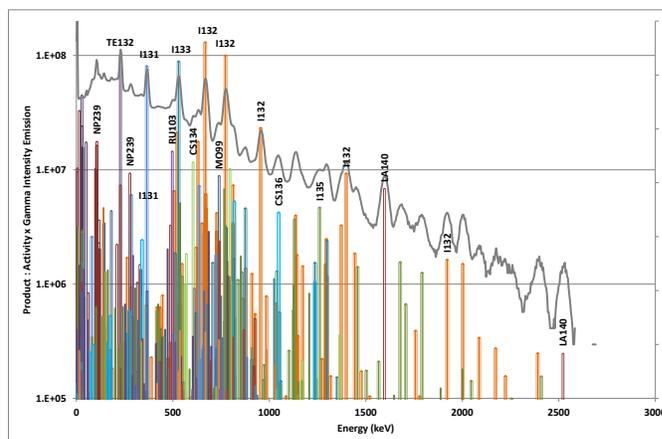
Fig. 4. Gamma spectrum modelled with a LaBr<sub>3</sub> detector in sight of the proposed aerosol device for the upper boundary scenario
