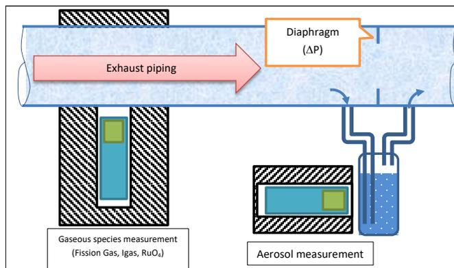
Fig. 3. Aerosol measurements on a trapping media in derivation to the main pipe
