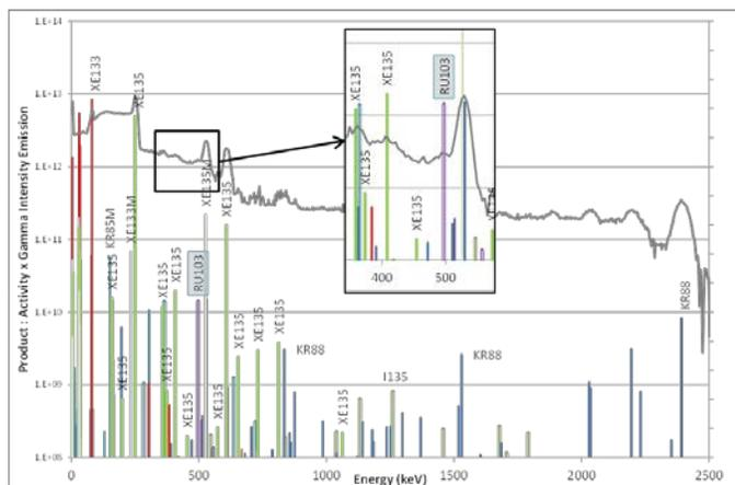
Fig. 2. Gamma spectrum modelled with a LaBr<sub>3</sub> detector for the upper boundary scenario at the outlet of the sand bed filter
