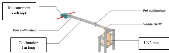
Fig. 1. Gamma spectrometry on the Megafox bench
