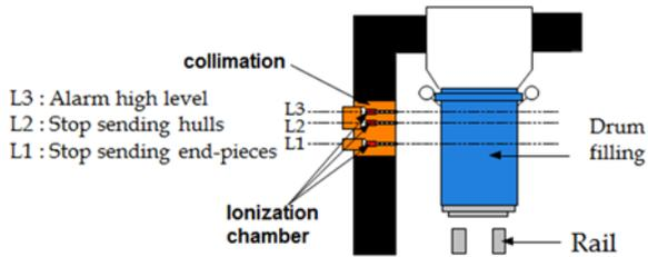
Fig 8. Schematic principle of the station 4 (first representation) based on the gamma-ray transmission measurement with two sources of  $^{60}\text{Co}$  and ionization chamber, the stations 5 (second representation) and 6 (third representation) based on the gamma-ray dose rate measurement with ionization chambers.
