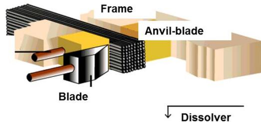
Fig. 2. Schematic principle of the shearing set-up.
