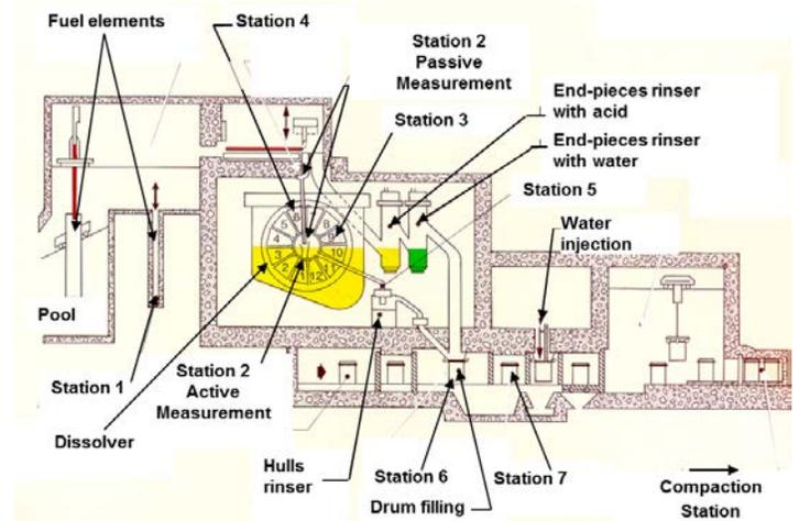
Fig. 1. Schematic principle of the process nuclear monitoring
