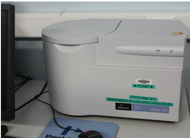
Fig. 3. Picture of the screen scanning device "Cyclone Plus" by Perkin Elmer; scanning time at worst resolution (169 \mu\text{m} ) is 4 minutes
