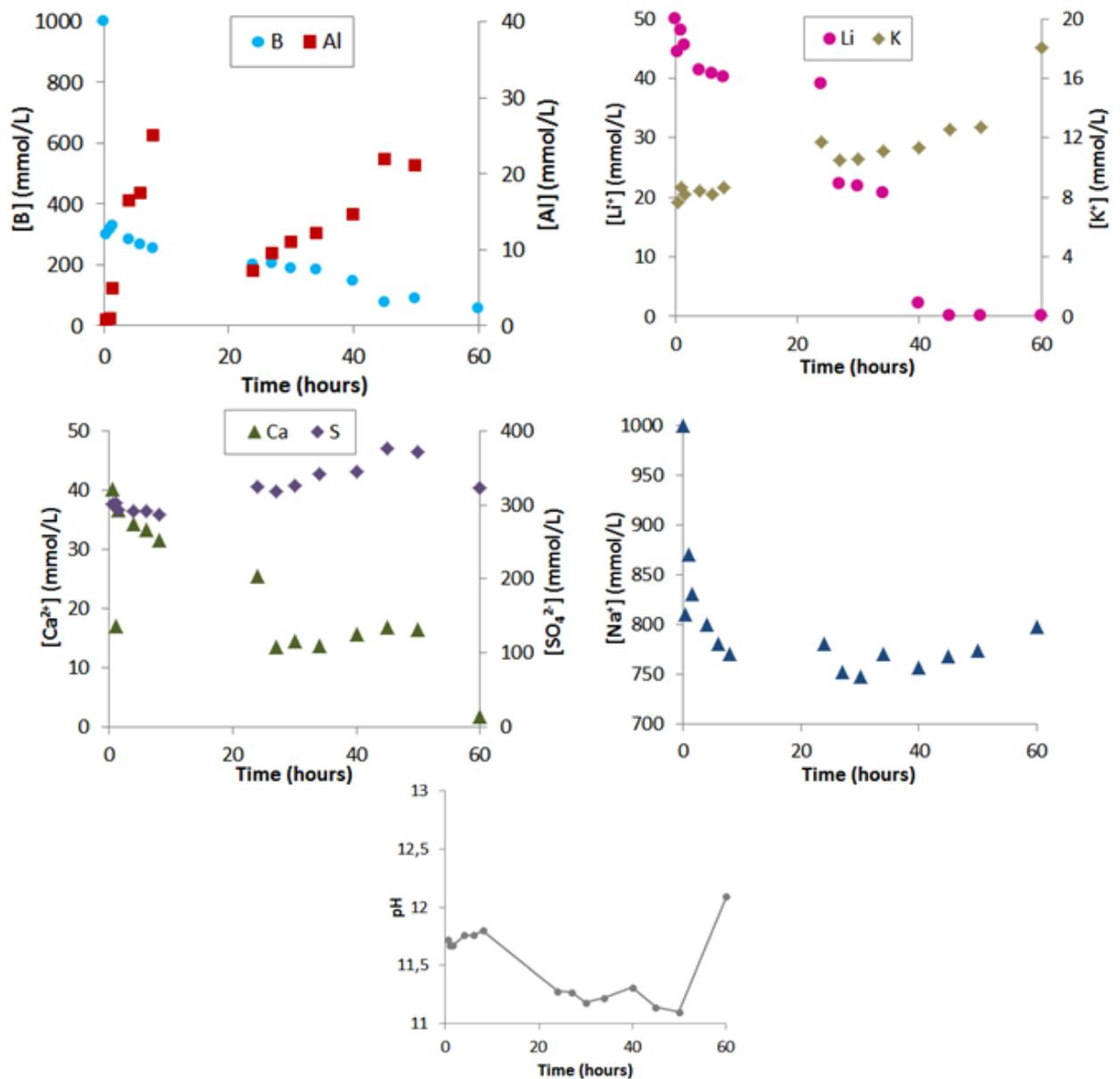
Figure 11 Hydration of CSA cement by a lithium/sodium borated solution ( $[B]_{tot} = 1 \text{ mol/L}$ ,  $Li/C = 0.03$ ,  $pH = 11$ ,  $w/c = 0.6$ ,  $T = 20^\circ\text{C}$ ) at an early age: evolution of pH and composition of the pore solution during hydration
