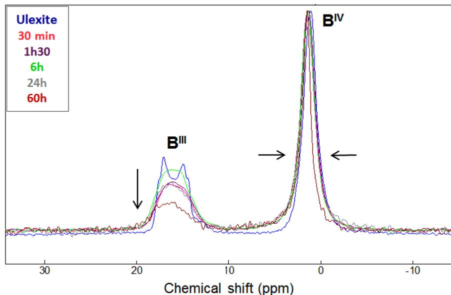
Figure 12 Comparison of the  $^{11}\text{B}$ -MAS NMR spectra of synthetic well-crystallized ulexite and of cement pastes hydrated by a sodium and lithium borated solution ( $[\text{B}]_{\text{tot}} = 1 \text{ mol/L}$ ,  $\text{Li/C} = 0.03 \text{ mmol/g}$ ,  $\text{pH} = 11$ ,  $w/c = 0.6$ ,  $T = 20^\circ\text{C}$ )
