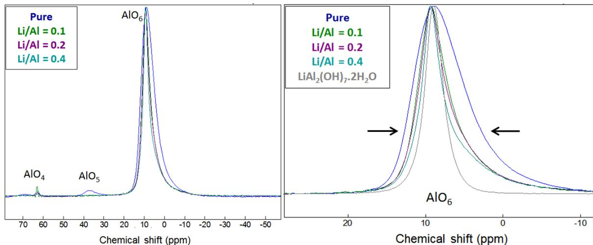
Figure 5  $^{27}\text{Al}$ -MAS NMR spectra of aluminum hydroxide (synthesized in the absence and in the presence of lithium) and of hydrated lithium aluminate  $\text{LiAl}_2(\text{OH})_7 \cdot 2\text{H}_2\text{O}$
