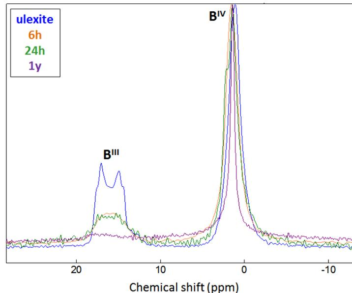
Figure 8  $^{11}\text{B}$ -MAS NMR spectra of ulexite and of cement paste samples hydrated by a sodium borate solution after 6 h, 24 h and 1 year. ( $[\text{B}]_{\text{tot}} = 1 \text{ mol/L}$ ,  $\text{pH} = 11$ ,  $w/c = 0.6$ ,  $T = 20^\circ\text{C}$ )
