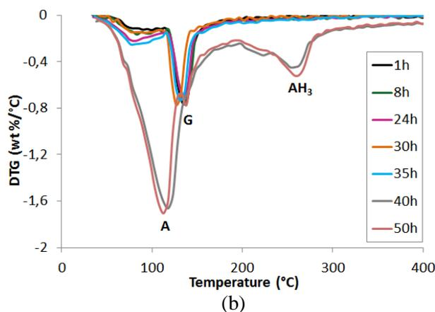
Figure 10 Hydration of CSA cement by a lithium/sodium borated solution ( $[B]_{\text{tot}} = 1 \text{ mol/L}$ ,  $\text{Li/C} = 0.03 \text{ mmol/g}$ ,  $\text{pH} = 11$ ,  $w/c = 0.6$ ,  $T = 20^\circ\text{C}$ ) at an early age : (a) X-ray diffraction patterns (A = AFt phase, G = gypsum, Y = ye'elimite, Si = silicon); (b) TGA analyses (A = AFt phase, G = gypsum,  $\text{AH}_3$  = aluminum hydroxide)
