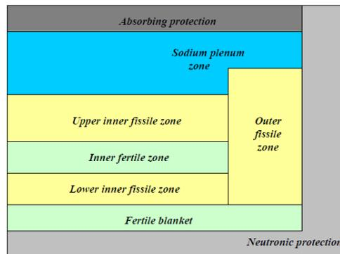
Figure 1: CFV general core geometry (radial cut)
