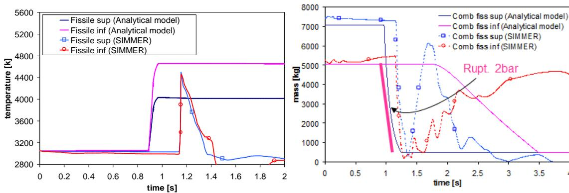
**Figure 7: Fuel temperature and mass evolutions in the lower pool of each fissile zone (comb: fuel, sup:upper; inf:lower)<sup>6</sup>**
