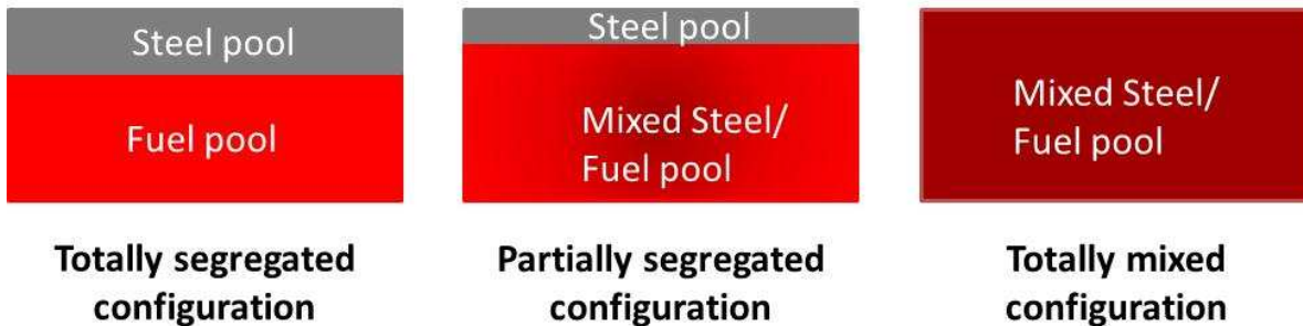
Figure 4: Various configuration of material repartition inside the upper or lower fissile zone.
