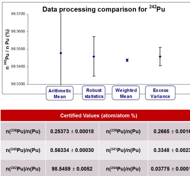
Fig 2: <sup>242</sup>Pu certification results
