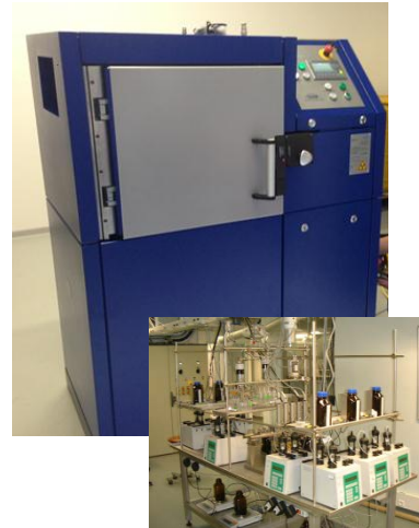
Fig. 15. Pictures of the new \gamma cell irradiator coupled to a process loop used to test the irradiation resistance of new extracting systems for Pu and U separation.
