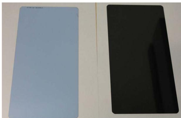
*Figure 1*: Phosphor screen used in the study; left: sensitive side, right: back side; type: TR, commercialized by Perkin Elmer; size: 12.5 x 25 cm<sup>2</sup>
