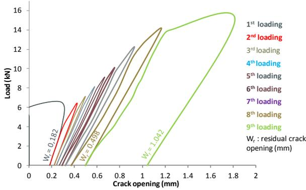
**Figure 5: Range of the residual crack opening obtained by the three point bending test**
