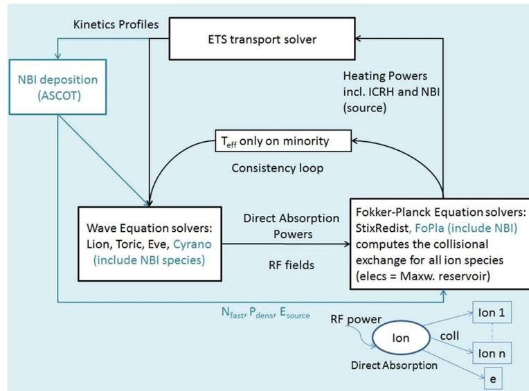
FIGURE 1: Sketch of ICRH-NBI Synergy Modelling in ETS
