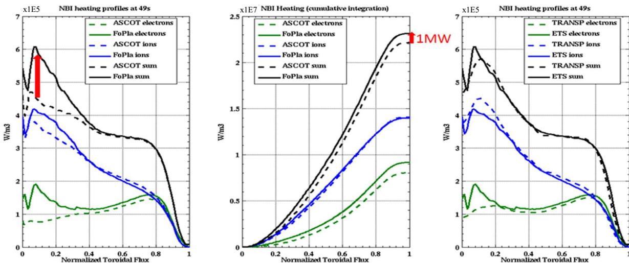
a) Comparison between ETS (ASCOT) without synergy and ETS (ASCOT/CYRANO/FOPLA) with synergy      b) Cumulative integrals.      c) Comparison between ETS and TRANSP
