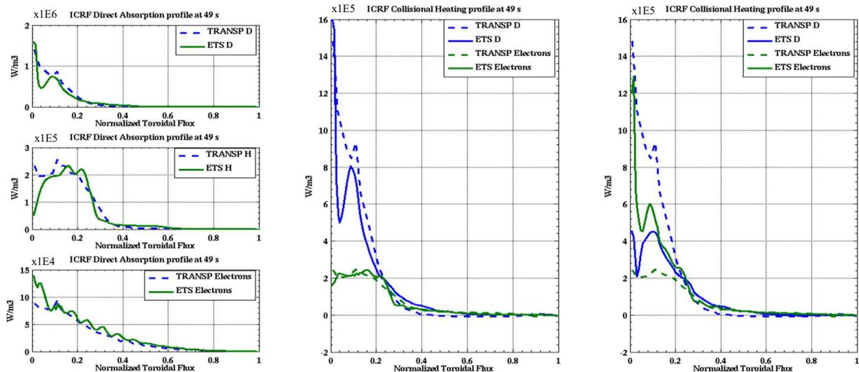
a) Direct ICRH power absorption profiles per species      b) Collisional power redistribution computed for H minority ICRF heating similar method use as in TRANSP      c) Full StixRedist calculation with non-linear H, D and self-collisions
