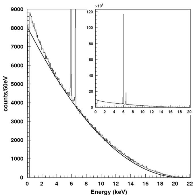
Fig. 2. Experimental and theoretical spectrum of  $^{241}\text{Pu}$ , using the Mn  $K\alpha$  line for energy calibration. The inset shows the full spectrum with the unclipped Mn  $K\alpha$  and  $K\beta$  lines.
