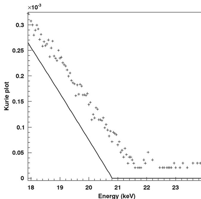
Fig. 3. Kurie plot of the region around the endpoint of the experimental (crosses) and the theoretical (solid line) spectrum of  $^{241}\text{Pu}$ , using the Mn  $K\alpha$  line for energy calibration.
