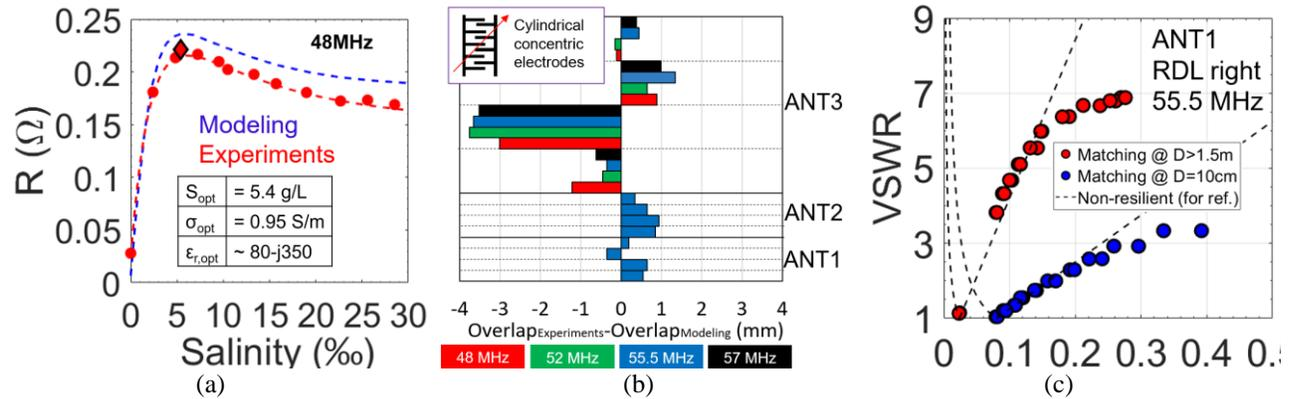
**FIGURE 4.** (a) Optimization of the dissolved salt concentration (numerical modeling is detailed in [11]). (b) Agreement of the measured capacitors’ electrodes overlap with modeling for the three launchers. Overlap measurements have been performed at several frequencies for ANT3. (c) Validation of the load-resilience in low-power experiments. R is changed by sweeping the launcher to load gap (D).
