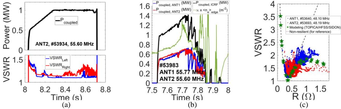
**FIGURE 6.** (a) 1 MW of coupled power with ANT2. (b) The ICRF power achieved 1.4 MW / 2 launchers just before a plasma crash. (c) The demonstration of the load-resilience on plasma and agreement with modeling. The non-resilient case is shown for reference. Numerical modeling is detailed in [11, 20, 21].
