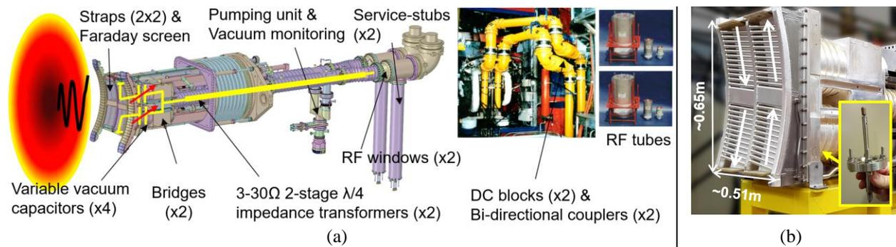
**FIGURE 1.** (a) Illustration of a WEST ICRF sub-system. The service-stubs allow injecting water-cooling pipes into the inner conductors. The length of the service stubs is about quarter-wavelength at 55 MHz. A Resonant Double Loop (see next section) is sketched in yellow over the launcher's CAD view. (b) A picture of the front face of a WEST ICRF launcher. The arrows indicate the ideal RF current direction for a dipole configuration. The subplot is a picture of a D-dot voltage probe.
