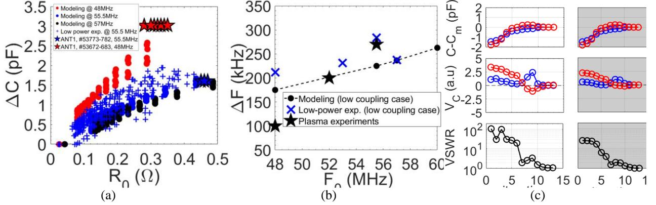
**FIGURE 5.** (a&b)  $\Delta C$  and  $\Delta F$  of the manual tuning strategy (see text). Good agreement is observed with modeling. With these settings, the VSWR is less than 1.05 (resp. 1.2) in modeling and low-power experiments (resp. on plasma). (c) Validation of the automatic matching algorithm. White (resp. grey) shaded plots: experiments (resp. modeling).  $C_m$  is a capacitance value at the final iteration corresponding to matching.
