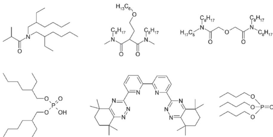
**Figure 1:** Extracting agents used in various GANEX flow-sheets: top, DEHiBA, DMDOHEMA, TODGA; bottom, HDEHP, CyMe<sub>4</sub>-BTBP, TBP.
