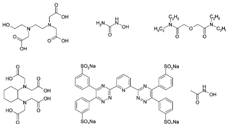
**Figure 2:** Water soluble complexing and reducing agents used in various GANEX flow-sheets: top, HEDTA, hydroxyurea, TEDGA; bottom, CDTA, SO<sub>3</sub>-Ph-BTP, AHA.
