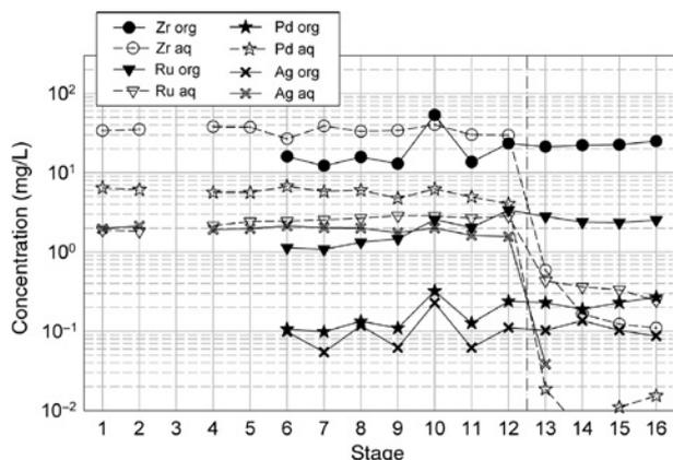
**Figure 10:** EURO-GANEX run, part 1 (preparation of loaded solvent), extraction (stages 1–12) and scrubbing (stages 13–16): Zr, Ru, Pd and Ag concentration profiles.
