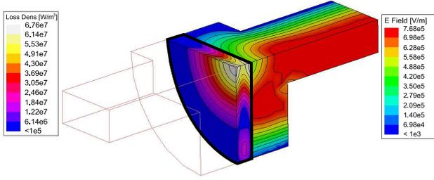
Figure 2: 3D view of the BeO window (1/4): The left colorbar represents the dielectric losses  $[W/m^3]$  inside the BeO ceramic for an input power of 500 kW. The ceramic has been underlined by a black line for clarity. The right colorbar represents the associated electric field in  $[V/m]$  in the vacuum section. 5 GHz ANSOFT HFSS simulation on matched ports.
