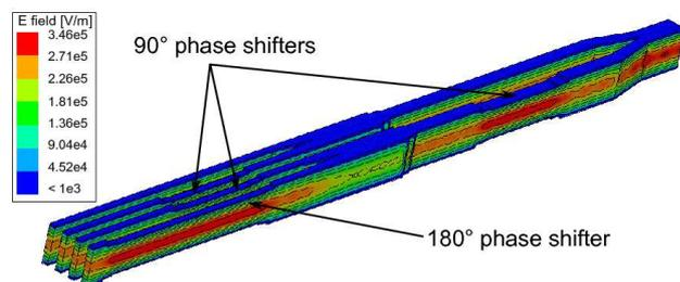
Figure 6: Electric field into the 4 active waveguides multijunction design. The input power is 83 kW, corresponding to the 250 kW incoming into the mode converter then divided by 3 in each rows of the poloidal divider. The passive waveguides located between each active waveguides are not illustrated in this picture. 5 GHz ANSOFT HFSS simulation on matched ports.
