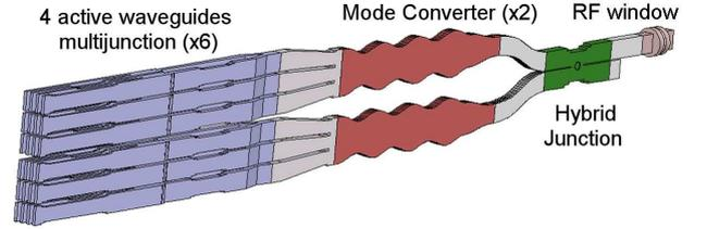
Figure 1: 3D view of one module (RF modeling): the power is coming from the right of the figure, through the RF window, the hybrid junction, the two mode converters and the six PAM multijunctions. All the elements of a module located behind the RF window are under the machine vacuum.
