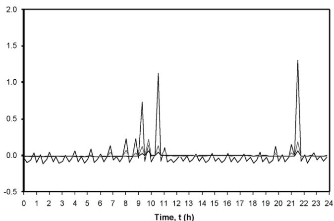
**Figure 2** Continuous monitoring of odour at the inlet of a sewage plant. The trace shows a 24 h recording using an array of four sensors sensitive to sulphurous odours. Odour events are recorded in real time and can be seen between 0800–1100 and 2100–2200 h.
