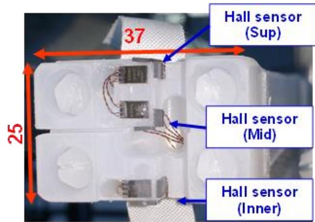
Fig2: Magnetic field sampler head used in experiment
