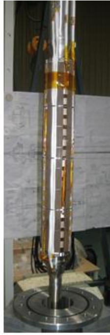
Figure 4 : The outer flask and the electromagnetic pump on the inner flask
