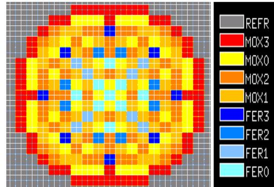
Fig. 3. Loading pattern of the HCPWR 19x19 core
