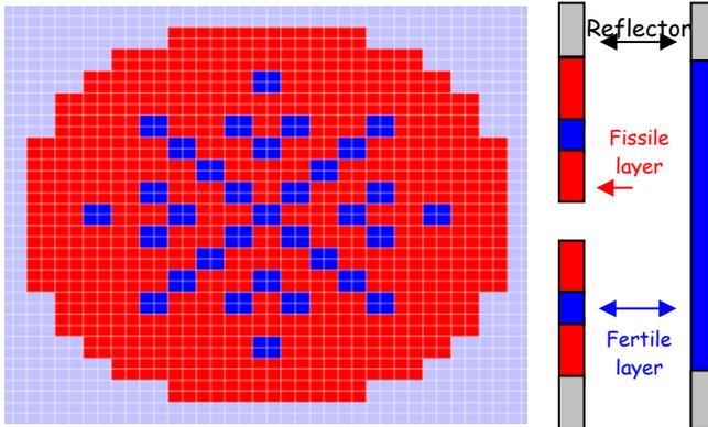
Fig. 2. Geometric description of the HCPWR 19x19 core
