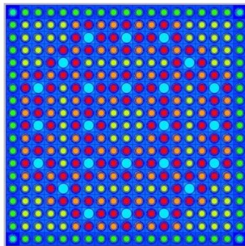
Fig. 5. Assembly Geometry used for depletion calculation
