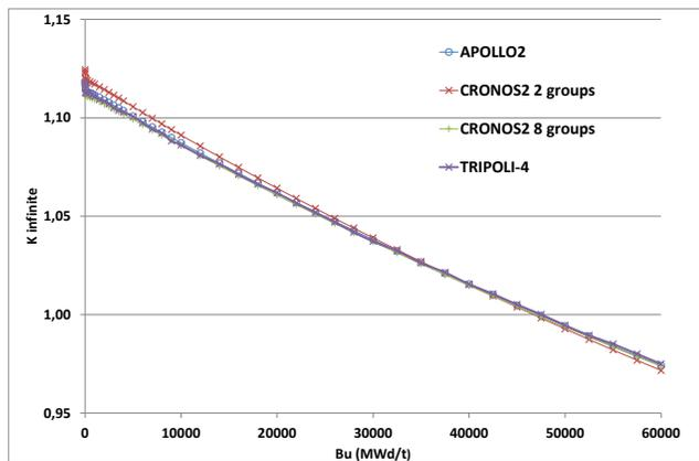
Fig. 6. Evolution of K infinity during depletion
