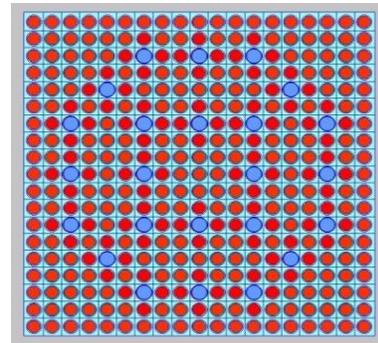
Fig. 1. Geometric description of the HCPWR 19x19 FA
