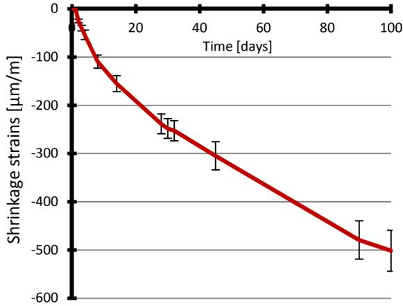
**Figure 3:** Experimental results of autogenous. shrinkage (mean and standard deviation).
