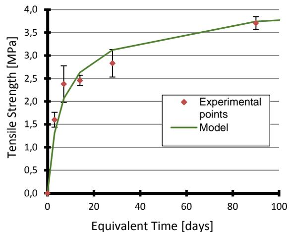
Figure 6: Modelling the evolution of tensile strength based on 3 points bending tests.
