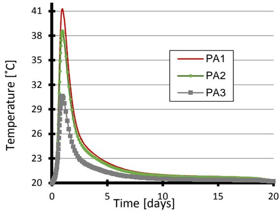
**Figure 9:** Temperature evolution in a massive activated slag mortar structure.
