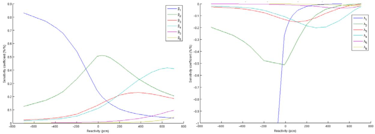
**Figure 2.** Sensitivity coefficients of the reactivity to  $\beta_i$  (left side) and  $\lambda_i$  (right side)
