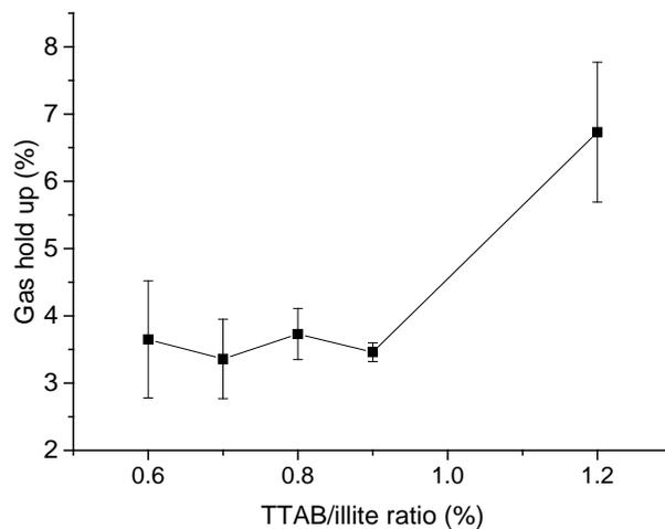
**Figure 6:** Evolution of gas hold up with the TTAB/illite ratio
