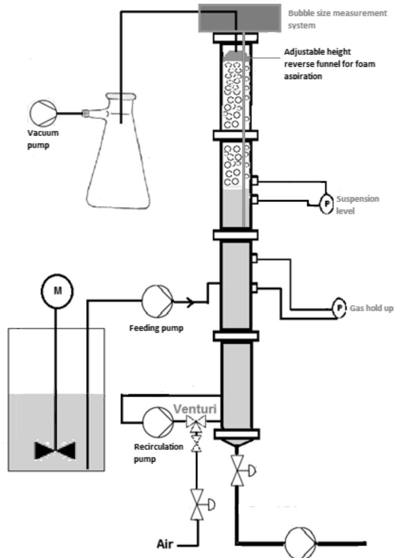
**Figure 1:** Schematic representation of the continuous flotation column
