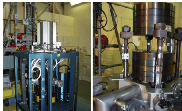
Fig. 1. CALIBAN reactor core (Left: core with cover; Right: the fuel core uncovered)
