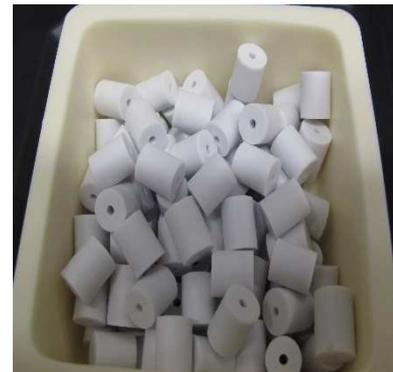
Figure 5 Sintered Al<sub>2</sub>O<sub>3</sub> pellets with hole
