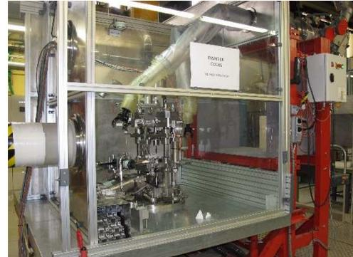
Figure 3 Press in mock-up for remote handling trials
