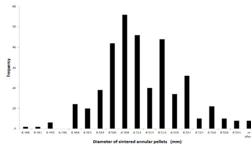
Figure 6 Histogram of the sintered pellet diameter
