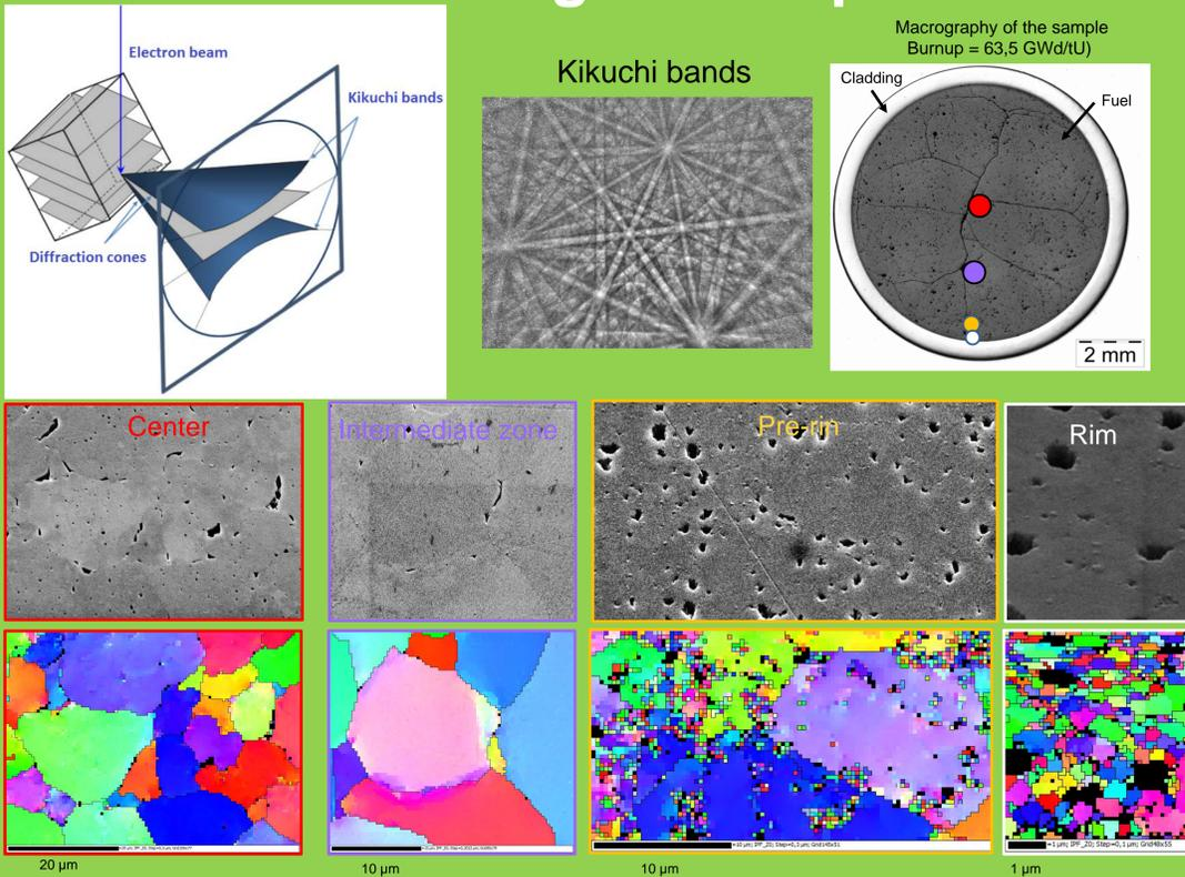
An irradiated UO<sub>2</sub> fuel was analysed by EBSD to observe the grains. Different radial positions in the fuel were studied : here, the center, the intermediate zone, the pre-rim and rim. The grain boundaries have been drawn for a misorientation superior to 10°. In the rim, the initial grains are subdivided in smaller grains.
