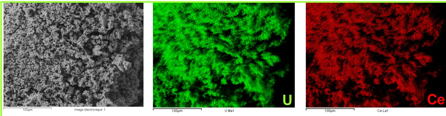
Energy dispersive spectroscopy revealed homogeneity of U and Ce distributions between microspheres.
