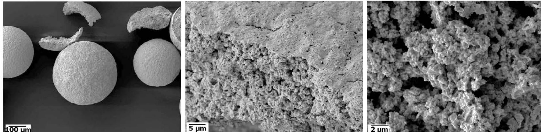
*SEM micrographs in secondary electron mode showing reduced oxide microsphere morphology and internal microstructure*
