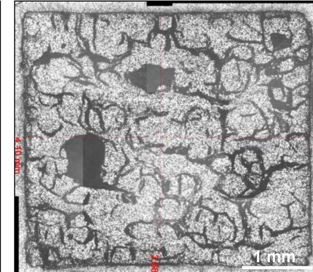
Interconnected hemispherical porosity => open porosity network
