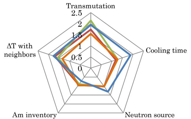
**Figure 7 : Radar plot showing the various impacts of the fissile material studied here. The red curve corresponds to <sup>235</sup>U, the green one to Pu<sup>239</sup>, the orange one to Pu 2035 and the blue one to the moderated case using ZrH<sub>2</sub>.**
