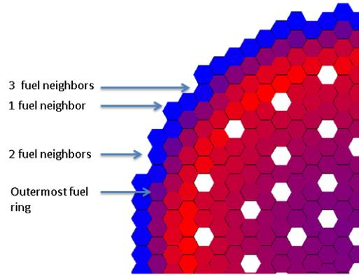
Figure 5 : Position of the various MABB assemblies considered
