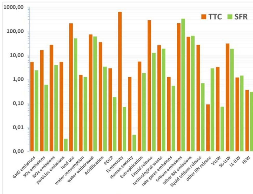
Fig.2: respective environmental indicators for the current TTC (mono-recycling of Pu as MOX fuels in current 2<sup>nd</sup> generation LWR) and SFR (multi-recycling of Pu in MOX fuels in Sodium Fast neutrons Reactors).
