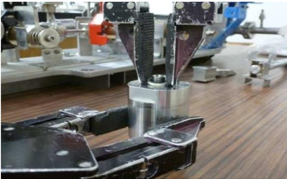
Fig. 2. Pressure gauge seal replacement by remote-handling
