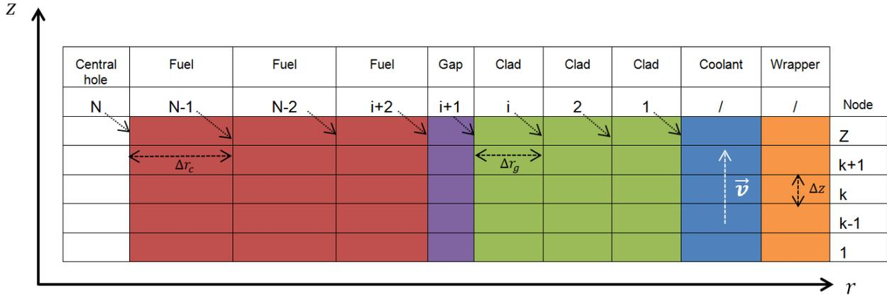
Figure 3. 2D meshing used for the modeling.
