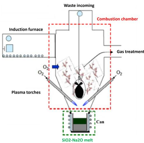
The **technological waste** coming from the production of uranium and plutonium Mixed Oxides fuel (MOx) results **contaminated** by  $\alpha$ -emitters and has to be treated as a long-life medium-activity nuclear waste. Treatments are then needed to fix the radio-isotopes in a stable matrix, in order to avoid an accidental release in the environment.
