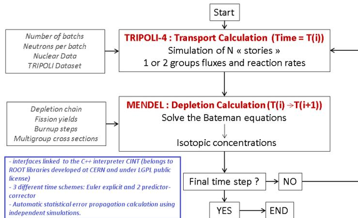
**Figure 3.** TRIPOLI-4<sup>®</sup>D architecture
