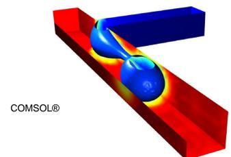
Fig. 4 : CFD simulation of multiphase flow in a T-junction Video accessible online at : [https://www.comsol.fr/model/download/11070/droplet\\_breakup.swf](https://www.comsol.fr/model/download/11070/droplet_breakup.swf)
